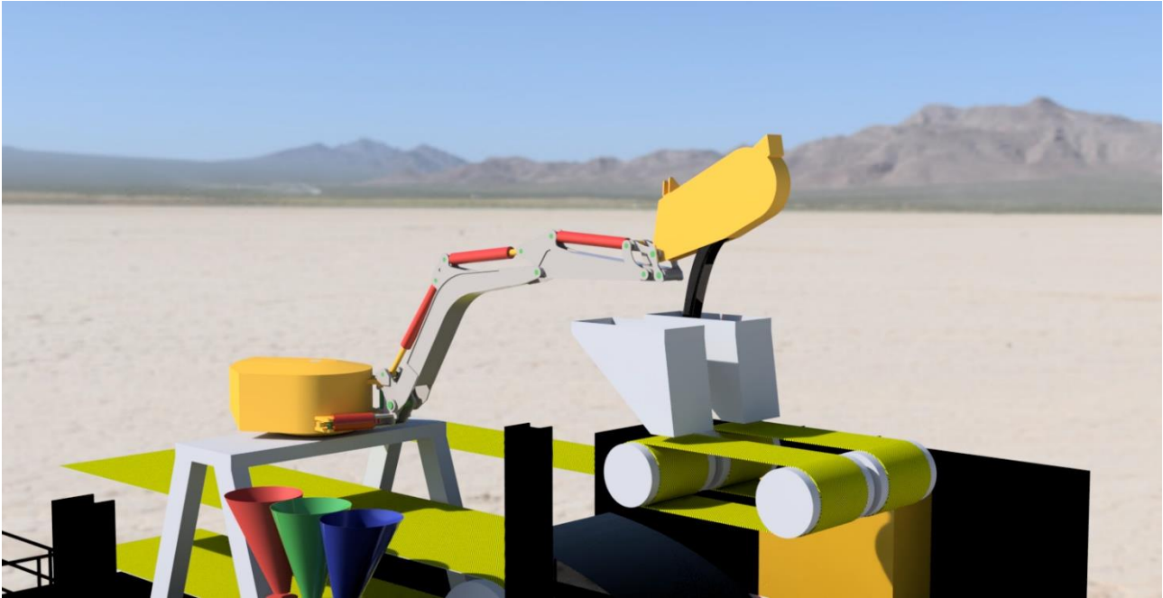
Fig. 3 – Uni-Samp feeding hopper for ‘feedback’ falling stream secondary sampling with same cutter.
